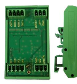
This output adapter converts the low-side digital outputs of the Baby-LIN-RM to high-side digital outputs. These high-side outputs are usually required by PLCs.
