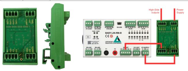
This output adapter converts the low-side digital outputs of the Baby-LIN-RM-III to high required by
