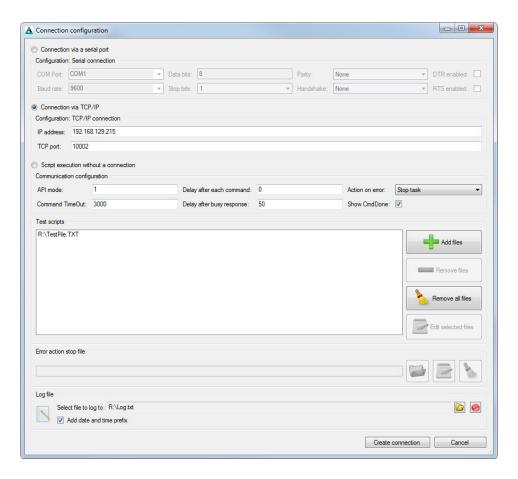
First choose a connection type (Serial, TCP/IP, no connection) and configure it.
