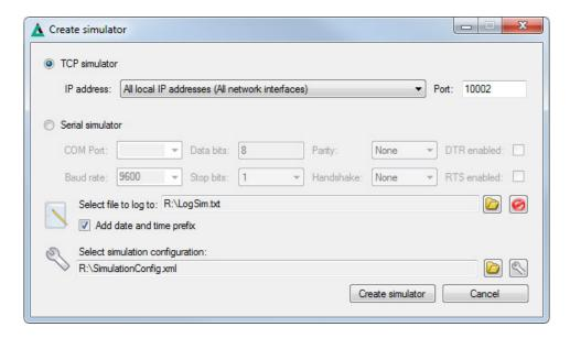
First configure the connection the simulator will handle. At the bottom you can select a simulation configuration file and edit it, by pressing the wrench button.
