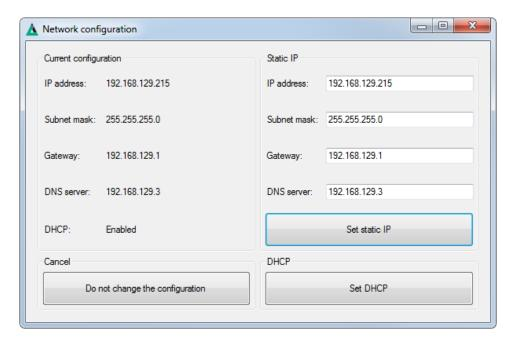
You can either enter the static IP data and commit the changes by pressing the "Set static IP" button or you simply press the "Set DHCP" button. In the latter case the network configuration will be received from a DHCP server.
