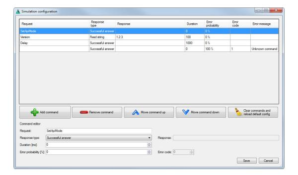
In this dialog you can edit the commands you want the simulator to react to. If your configuration is empty, you can load a minimal configuration by pressing the "Clear commands and reload default config" button.
