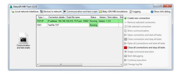
The table shows you all configured devices and test scripts no matter if running or not. A device line uses the following column headers:
