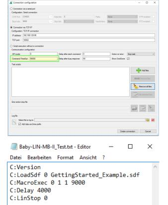
The script is executed by clicking on the "Open connection and start all tasks" button. The test script execution view can be opened by double clicking on the connection.
