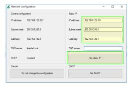
Make sure that your PC has a network interface available to access the same subnet. If the parameters are set up correctly you should be able to open the device webpage by clicking on the earth icon
