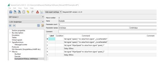
A macro can receive up to 10 parameters when called. In the macro definition, you can give these parameters names, which are then displayed on the left in the menu tree in brackets after the macro name. The parameters end up in the signals \_LocalVariable1...10 of the called. If no parameters or less than 10 parameters are are passed, the remaining \_LocalVariableX signals receive the value 0.
