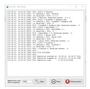
After running the SDF macro in Stand alone mode with BabyLIN MB-Tool pc software you now can replace the BabyLIN MB-Tool by your PLC and send the commands from there.
