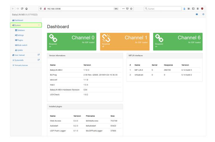
The dashboard in stand alone mode can be used to check the correct wiring of the LIN bus power supply. LIN bus and LIN bus supply (12V) are connected to X9.
